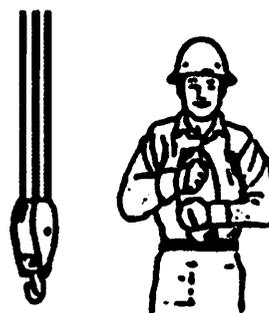
**TRAVEL (Both Tracks).** Use both fists in front of body, making a circular motion about each other, indicating direction of travel, forward or backward (for land cranes only).
