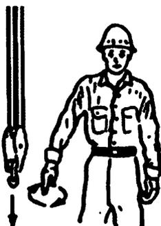
**LOWER.** With arm extended downward, forefinger pointing down, move hand in small horizontal circles.
