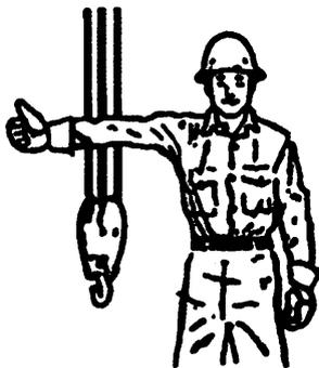
**RAISE BOOM.** Extend arm, fingers closed, thumb pointing upward.
