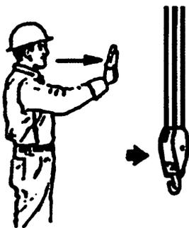
**TRAVEL.** Extend arm forward, hand open and slightly raised; make pushing motion in direction of travel.
