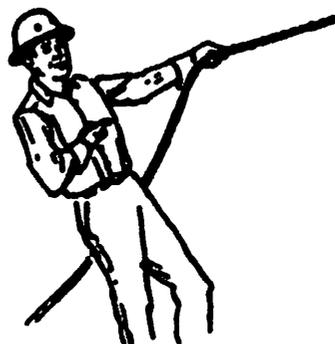
**RETRACT BOOM (Telescoping Boom).** One-hand signal. Hold one fist in front of chest, thumb pointing outward and heel of fist tapping chest.
