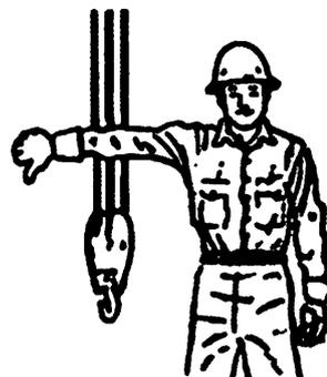
**LOWER BOOM.** Extend arm, fingers closed, thumb pointing downward.
