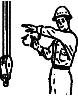
**MOVE SLOWLY.** Use one hand to give any motion signal and place other hand motionless above the hand giving the motion signal. (Hoist slowly shown as example.)
