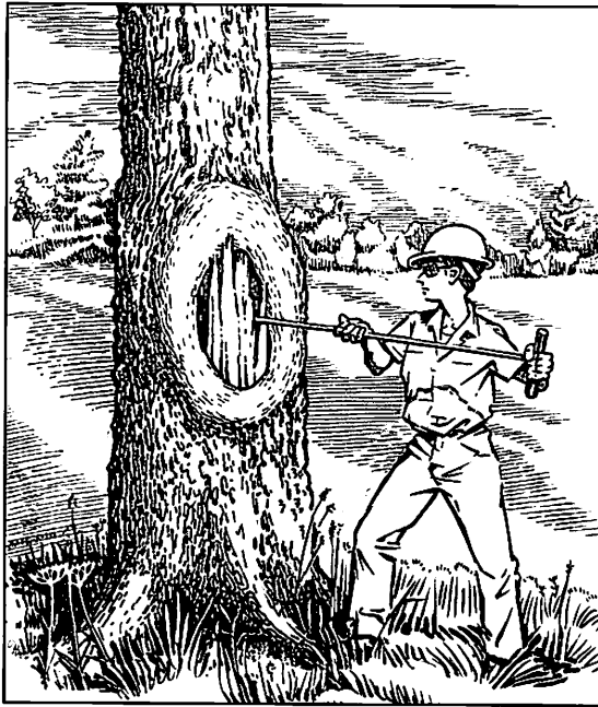
Figure 2. Probing. The tree risk assessor can use a stiff, small-diameter rod or stick to probe into cavity openings to estimate their size and extent.
