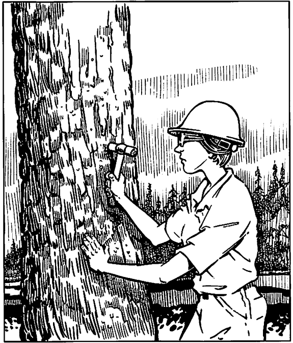
Figure 1. Sounding. The tree risk assessor can strike the tree with a mallet and listen for tonal variations that indicate dead bark or internal hollows.
