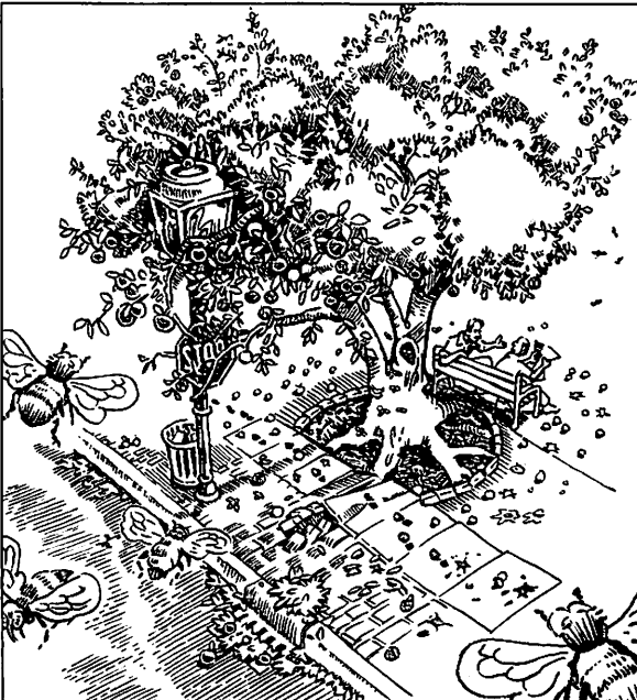
Figure A1-1. Conflicts result when trees interfere with people, property, or activities and may result in harm. In this case, conflicts include attraction of stinging insects, falling and fallen fruit, pavement lifting, interfering with street lighting, and blocking visibility of the stop sign.
