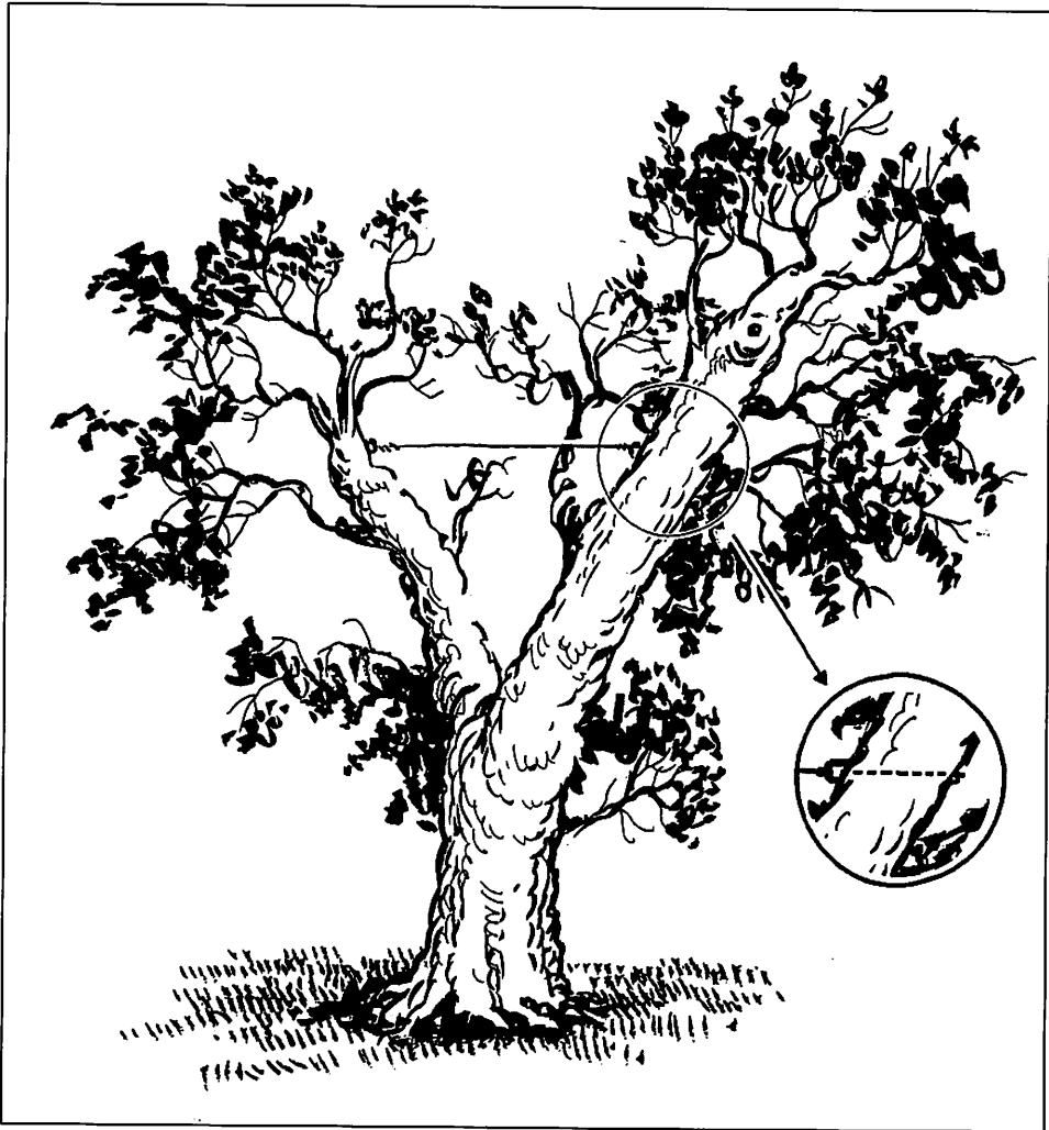
Figure 13. Anchor hardware must be installed in direct line with the cable to ensure maximum strength of the system.
