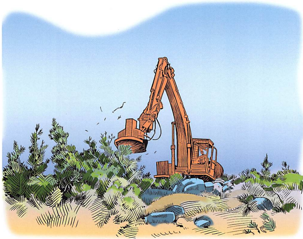
Figure 6. Masticator mounted on an excavator.
